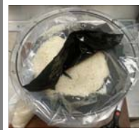
Figure 1: Since PRESAGE® is temperature and light sensitive, dosimeters were stored in a black, light-tight bag in a refrigerator at 4° C until irradiated. During irradiation, the PRESAGE® stayed in the black bag and was surrounded by rice, which was used as tissue equivalent material. 4
