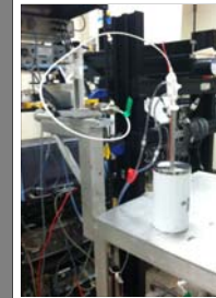
Figure 3: The Xoft Axxent catheter was plugged into the MTF. The catheter was then inserted into the cylindrical PRESAGE® dosimeters to irradiate them to 15 and 20 Gy.
