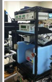
Figure 2: The Modulator Test Fixture (MTF) at the University of Wisconsin ADCL was used to mimic the Xoft Axxent Controller.
